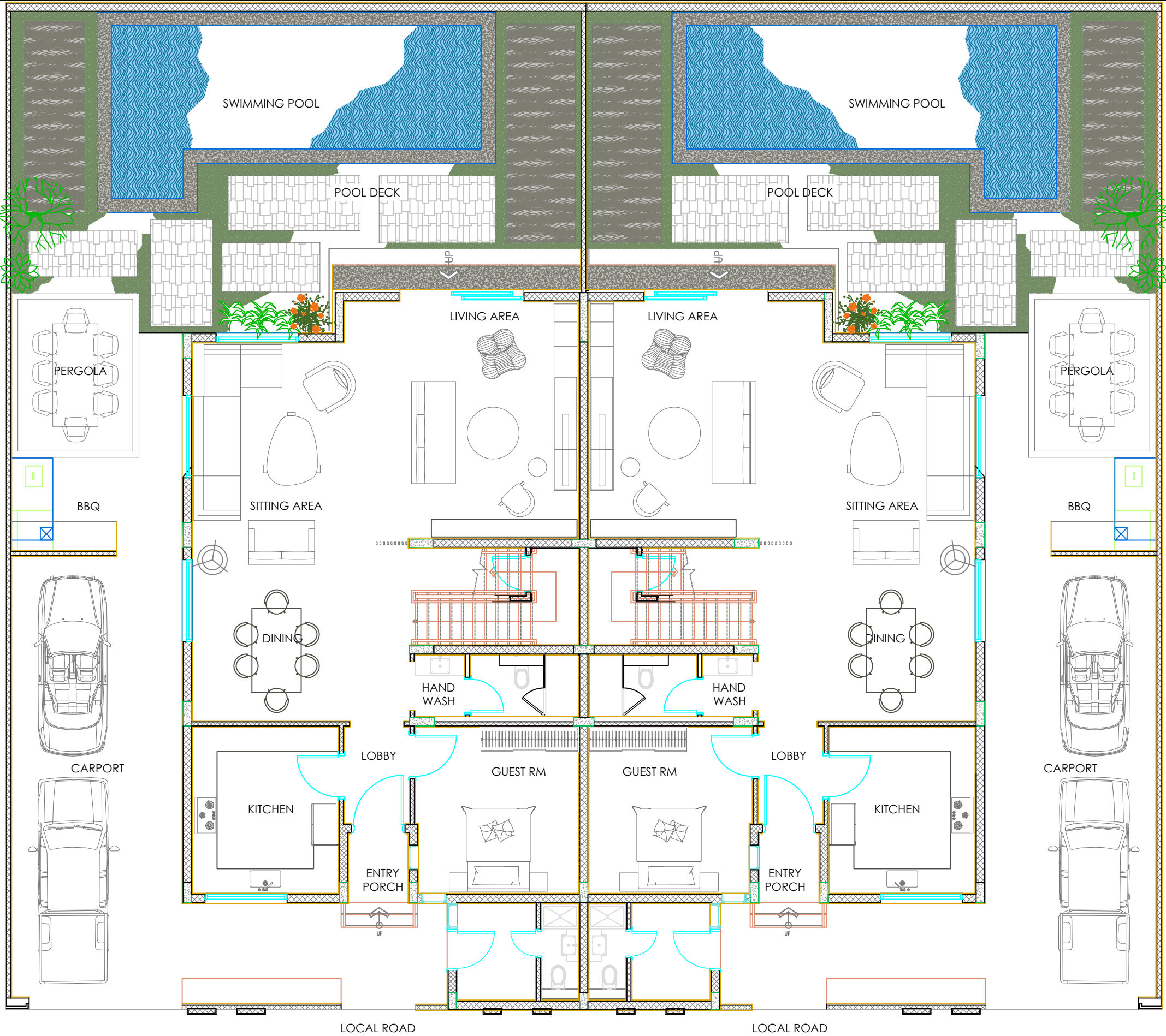
TYPE A DUPLEX - GROUND FLOOR GENERAL ARRANGEMENT 1 GA-01 SCALE 1:100
